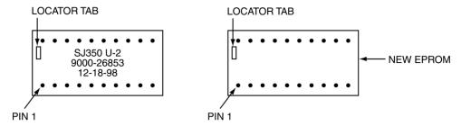
Note that the socket has a similar locator tab. Install the EPROM in the socket. This may require bending of the pins slightly as you guide them into the socket. When all of the pins have been started into the socket holes, seat the EPROM firmly into the socket. Inspect the EPROM for any bent pins and correct orientation of the locator tab.
