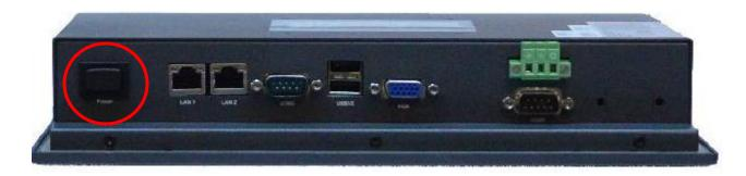
The power button is circled above, it is on the lower left when facing the screen. Pressing this when power is on will boot the PC if there are no other problems with the PC. To restore full functionality to the battery, keep the unit powered on for 24 hours.
