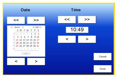
You must adjust the clock forward month by month with the ">>" button and the time with the "<" and ">" buttons. When the date and time are correct press the "Done" button
